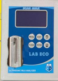
**Embedded function real date** and time-registers the exact time for delivery of milk in the milk collecting center
